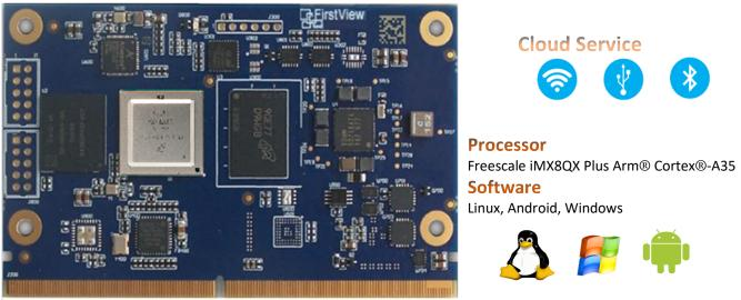
FirstView follows up on the success of i.MX6 and i.MX8X Series SOM offering with a rugged, reliable and low cost i.MX8QXPlus Version. The FVC-MX8QXPlus-SOM is an embedded single board module optimized for performance and power with a life cycle that removes concerns for obsolescence. The board is designed to be paired with a custom carrier board to fit specific applications in a wide range of environments.
